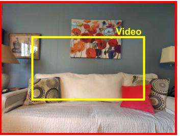
If the XREAL BP was just cropping the original frame, the resolution of the video frame would have been ~2560x1440 pixels. The camera resizes this to 1920x1080.
